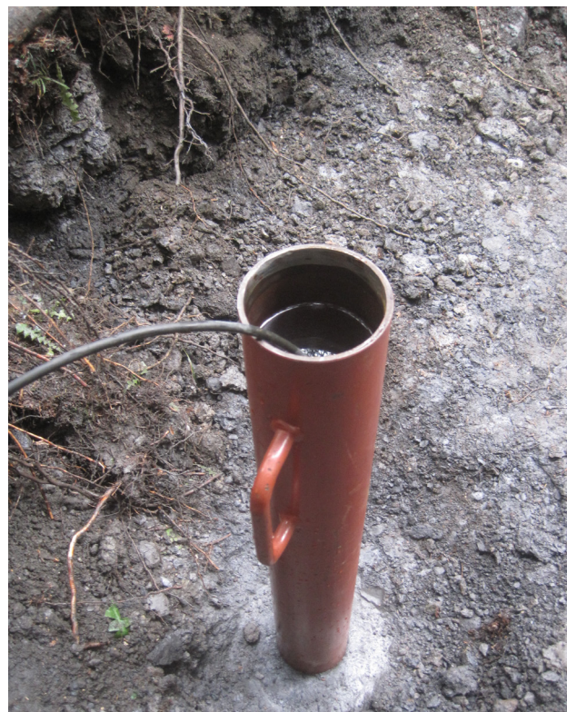
Fig. 4. Open-bottom tubes for performing falling-head test (photo: Zmago Bole).
