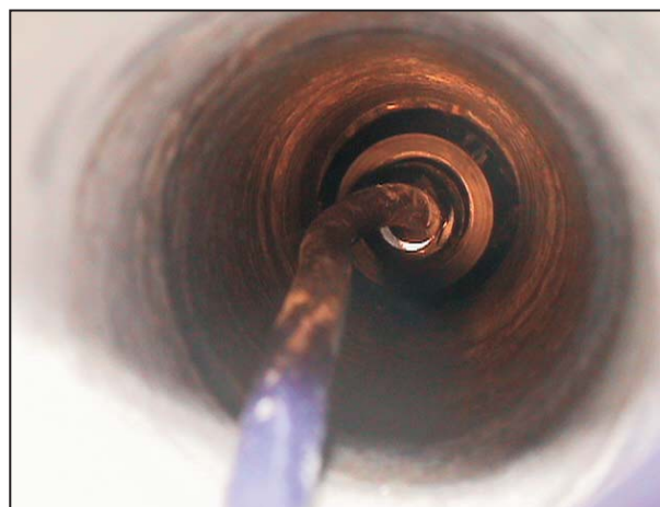
Figure 16., 17. VW Biaxial Stressmeter and its position in the borehole.
