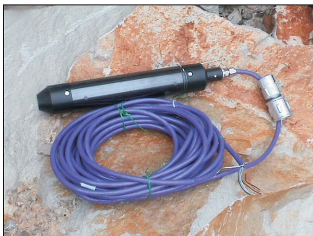
Figure 16., 17. VW Biaxial Stressmeter and its position in the borehole.
