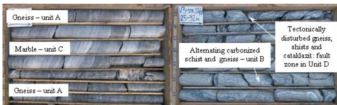
Figure 8. Most common lithological units in the area of the engine room.
