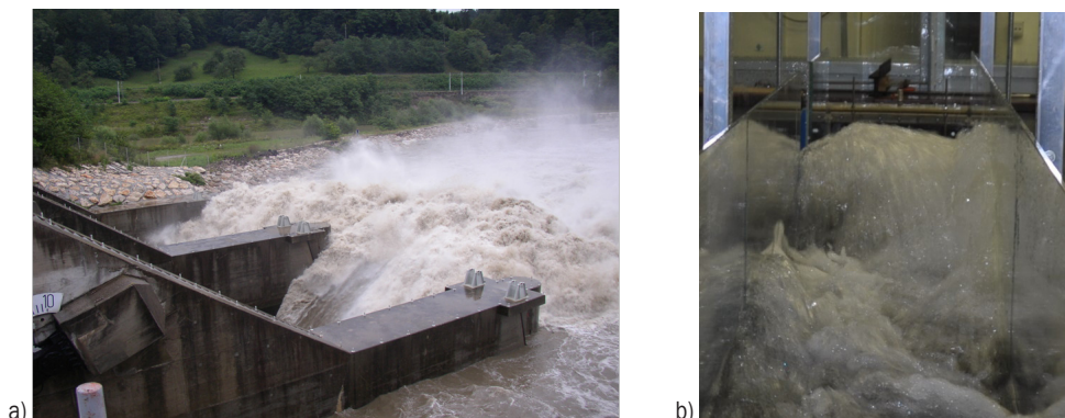
Fig. 1. a) The dynamic water surface below the Vrhuvo HPP, and b) the experimental apparatus at the hydraulic laboratory, where distinctly standing waves are formed at the confluence of two incoming supercritical flows
