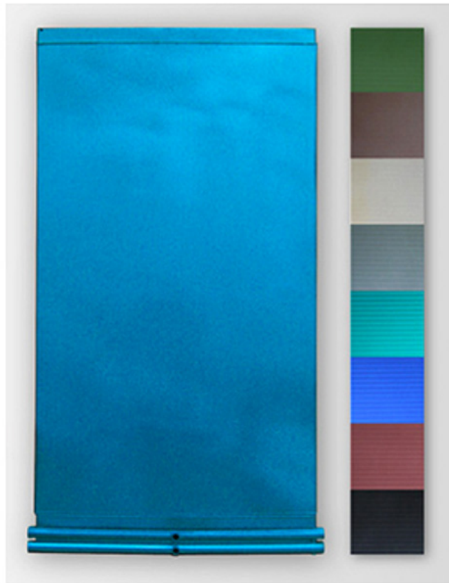
Figure 4. Absorber module (in PPS) of the AVENTA polymeric solar collector coated with blue selective paint and selection of coloured selective paint coatings made in the frame of the project.
