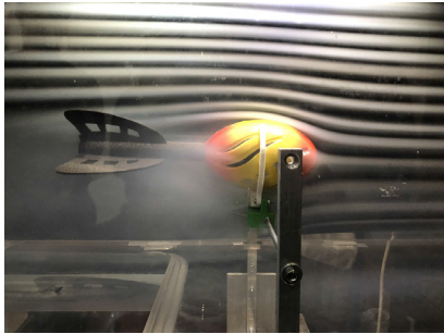
Fig. 22. Attack store during drag testing
