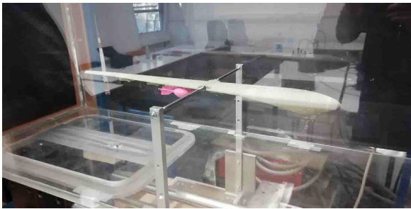
Fig. 23. Fuselage drag measurement in wind channel
