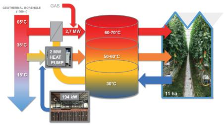
Special highly efficient Kronoterm heating and cooling system
