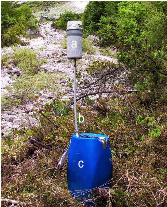
Figure 2: Specimen of a rain gauge: catching vessel with a funnel (a) connected to container (c) by means of a narrow tube (b) (photo: E. Kozamernik).
