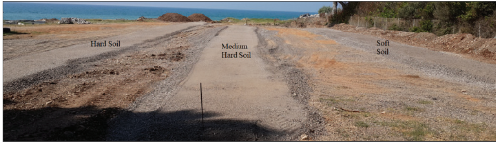
Figure 1. Preparation of soft, medium hard and hard soil pits for post installation.
