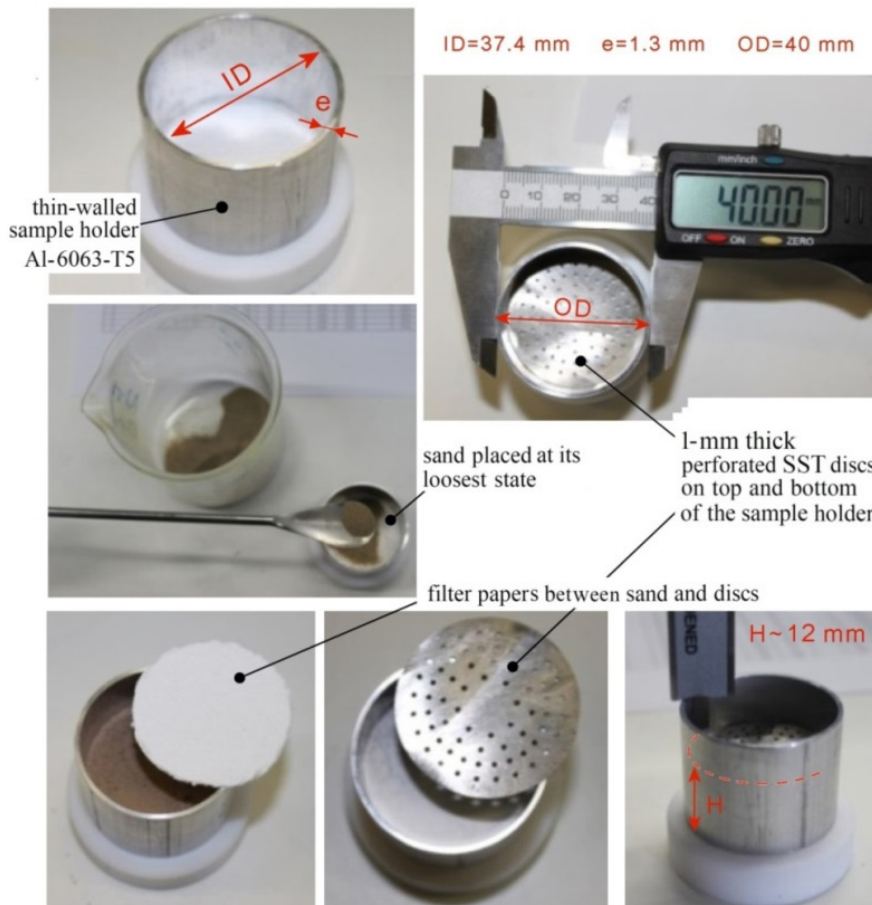
Figure 3. Sample preparation of the one-dimensional compression tests.
