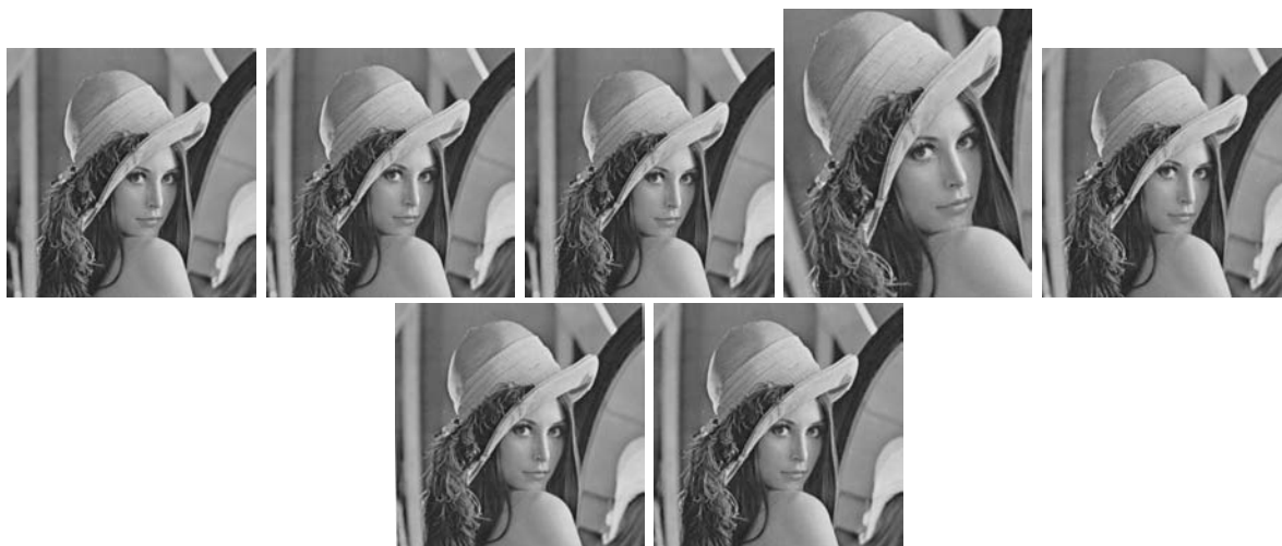
Figure 6: Left to Right, Top to bottom: (a) original Lena image, (b) watermarked Lena with random pre-warping, (c) watermarked Lena without random pre-warping, (d) scaled, rotated and cropped image, (e) StirMarked watermarked image, (f) marked image after shearing distortion, (g) re-watermarking of marked image.
