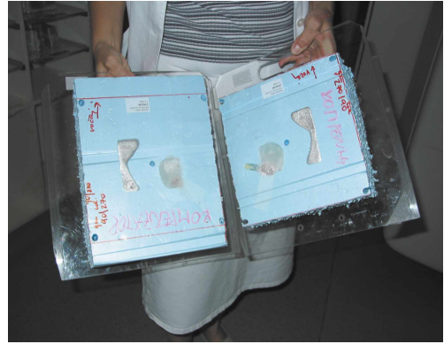
Figure 4. The foam blocks with blocking filters made of Wood alloy and filter compensators made of paraffin wax, were manufactured for each of the lateral opposed fields (gantries 270i and 90i). The central hole was drilled in each of the foam block in order to see the center of the optical fields. The positioning holes were drilled in the corners of the blocks. The 30 \times 30 \times 8 cm 3 foam blocks had to be cut to the suitable dimension for Philips SL 75/5 linear accelerator, i.e. to 21 \times 30 \times 8 cm 3 . The foam blocks were fixed on the positioning trays, ready to use.
