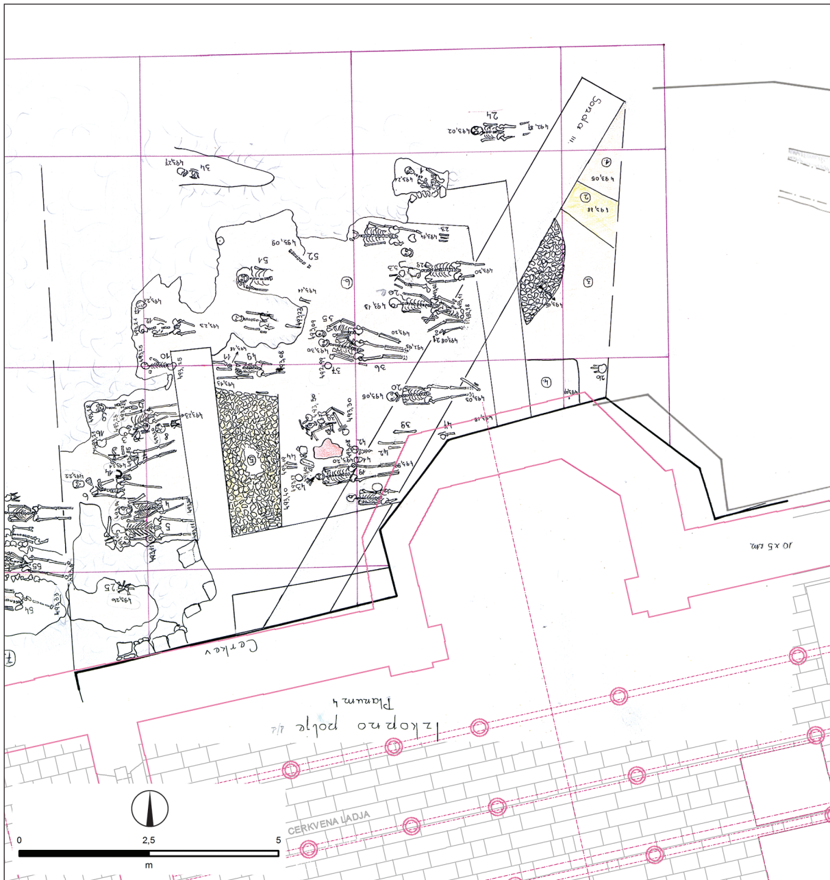
Fig. 5: Bled Island, plan drawings of the graves north of the present church, georeferenced with the grid reconstruction method. The residual error of georeferencing can be seen when comparing the modern plan of the present church (red) with two plans from the 1962–1964 excavation (black, grey); the plan drawing is oriented to the north.
