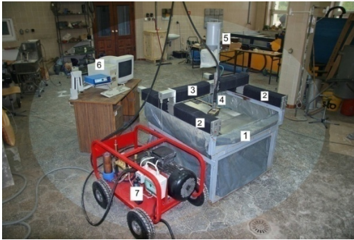
Fig. 2. A general view of test stand for spatial material machining with high pressure abrasive-water jet: 1) frame, 2) y direction slideways, 3) x direction slideway, 4) abrasive-water jet working head, 5) abrasive feed container, 6) steering PC computer, 7) high-pressure water pump type As500/15A
