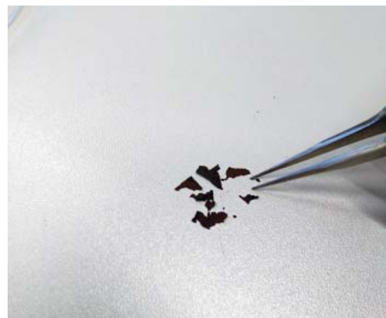
Figure 5: (a) Bending sample carbonised at 500 °C, electrospun from 1.6 g PAN and 0.2 g casein; (b) broken residues after the same bending test, performed on carbonised (500 °C) sample electrospun from 1.6 g PAN without casein
