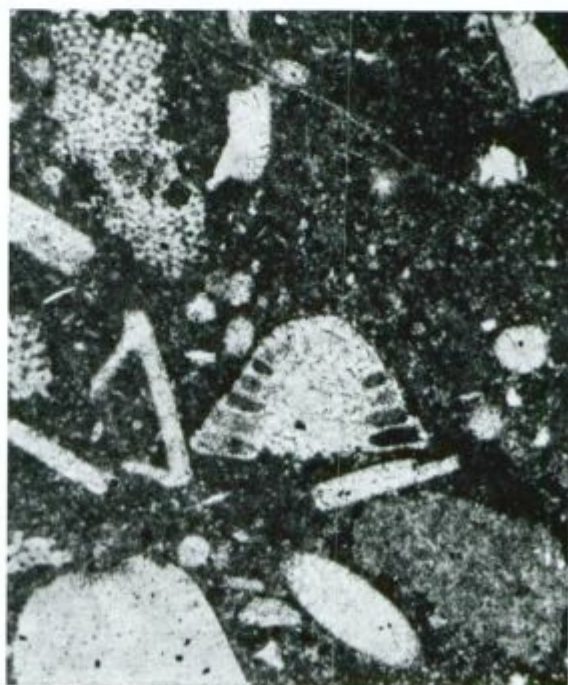
Sl. 6. Liasni laporasti mikritni apnec z vrsto Neoangulodiscus leischneri Kristan-Tollmann, Črni vrh, 43 × Fig. 6. Liassic marly micritic limestone with Neoangulodiscus leischneri Kristan-Tollmann from Črni vrh, 43 ×
