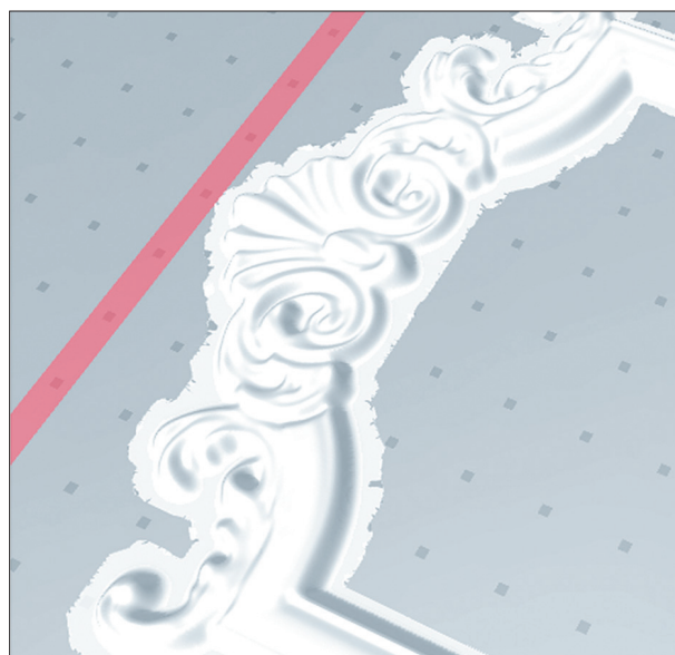
Slika 9. Tekstura STL modela pri desetih prehodih glajenja Figure 9. The texture of the STL model after ten smoothing passes
