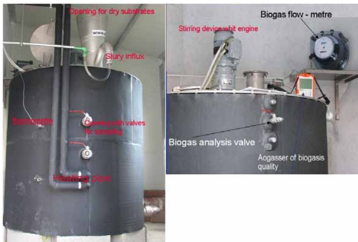
Figure 1: Test reactor (on the left: view from the front, on the right: view from the back). Slika 1: Preizkusni reaktor (levo: prednja stran, desno: zadnja stran).
