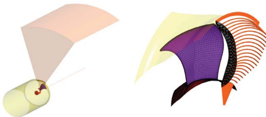
Fig. 7. Overall and detailed 3D calculation model of fan with the guard grill
