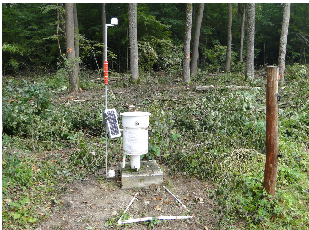
Fig. 4. Malence Borehole Temperature Observatory (in Sept. 2011). Sensors in the soil are buried within depicted trapeze.
