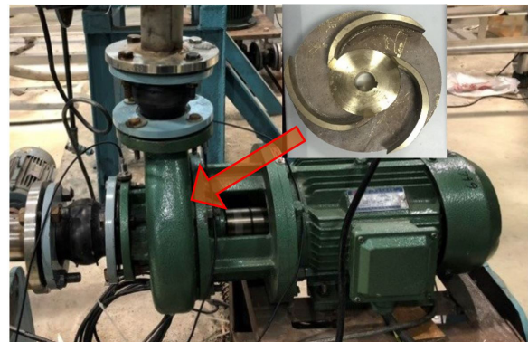
Fig. 1. Photo of the model pump with a cylindrical blade
