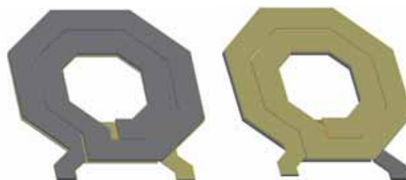
Fig. 9(b): 2-metal layer optimized inductor layout: light grey: metal 1, dark grey: metal 2.
