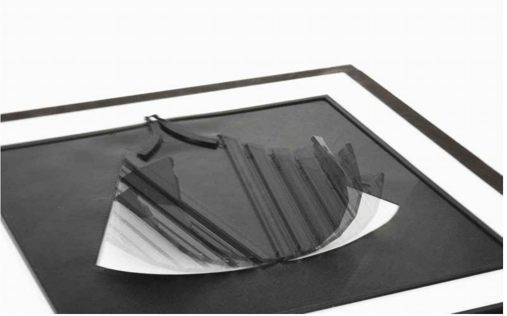
Figure 2: van Brummelen, Paula (November 2020): Movement of a surface structure with integrated Shape Memory alloy
