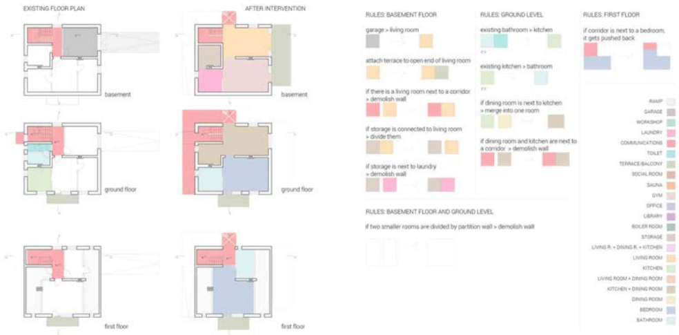
Figure 4: Determining the design rules based on the changes made to the floor plan – an example.
