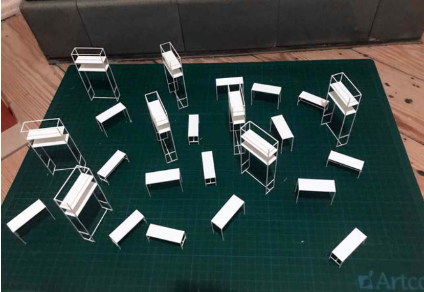
Figure 3: Initial explorations in 1:20 model. 3-dimensional enabling furniture system adapting to existing floor plans.
