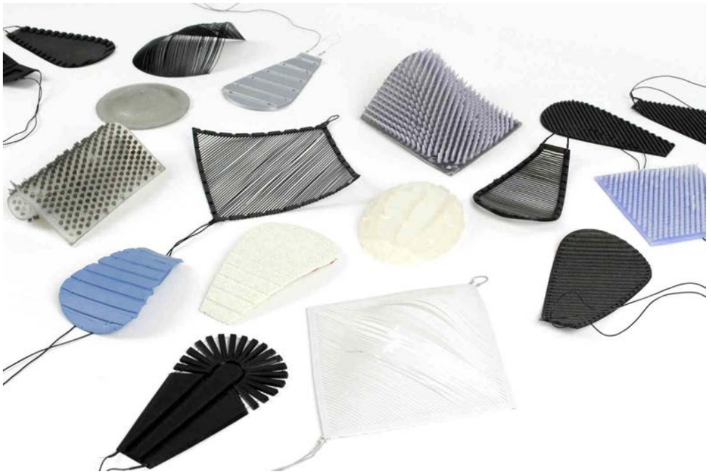
Figure 1: Material Experiments with kinetic functional Potentials. van Brummelen, Paula (December 2020): casted and 3d printed material experiments with kinetic functional potentials
