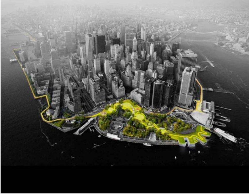
Figure 1: Artist's impression of The BIG U proposal. In the image it is visible the idea of the "active border", consisting in a sequence of public spaces, undulated berms, rain gardens, street furniture, pavilions, deployable walls and landform buildings which work both as a defence and an enhancement of the public realm. Source: https://big.dk/#projects-hud (accessed June 2021)
