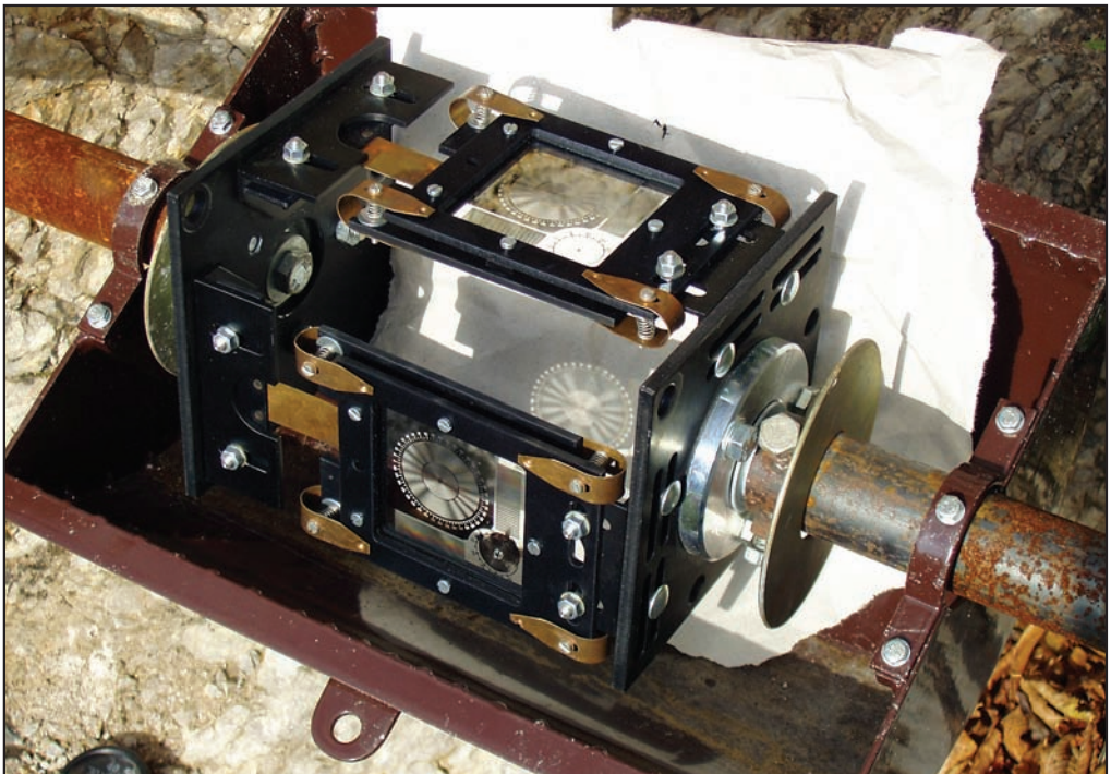
Figure 4: The TM 71 extensometer which measures tectonic micro-displacements in three directions.
