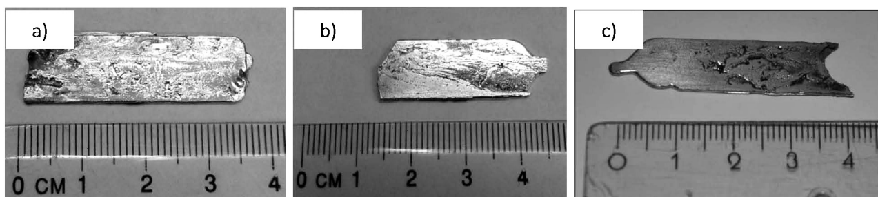
Figure 1: Three samples: a) sample 1, b) sample 2, c) sample 3, produced with the pressure-die-casting method
