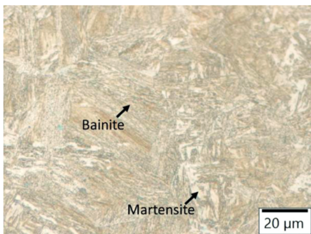
Figure 1: Typical microstructure of the HTCS-130 – 0 steel samples consisting of bainite and martensite (HTCS-130 – 0, quenched from 1060 °C)
