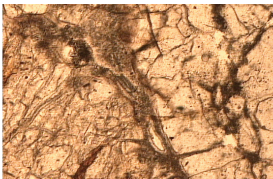
Figure 2: Metals in cracks of glaze: transmitted light, magnification 100 \times , one nicol.
