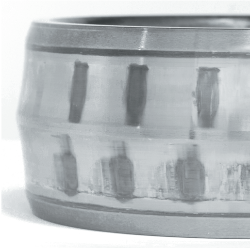
Fig. 10. Damaged bearing of lever pivot
