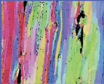
EBSD grain orientation map of Mo (Ti,Zr) alloy
