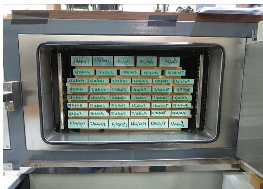
Figure 2. Experimental drying chamber with wood samples.
