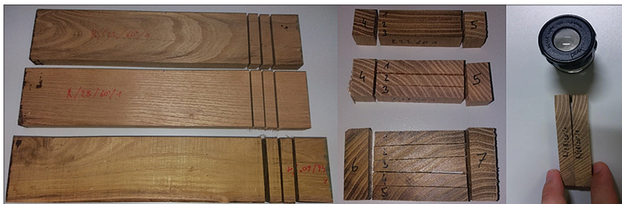
Figure 3. Samples for determination of the moisture content gradient and drying stresses.
