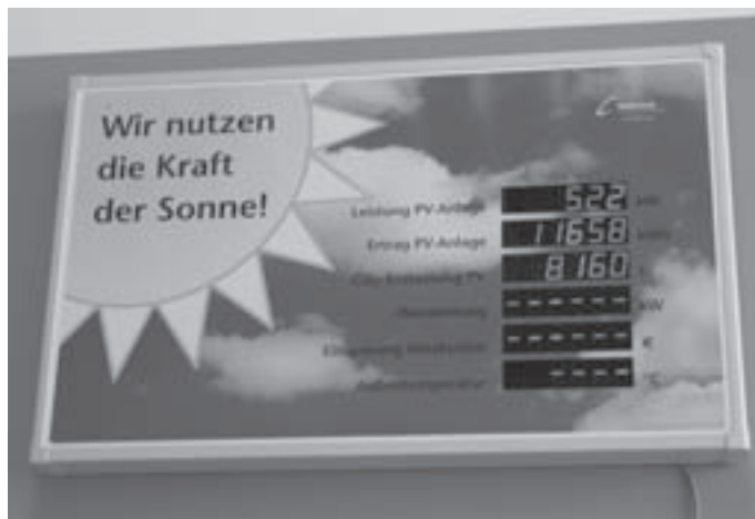
Slika 2: Na steni glavnega hodnika je mogoče ves čas spremljati količino pridobljene električne energije ter prihranek CO 2 . Figure 2: On the wall of the main corridor, it is possible at all times to follow the amount of electrical energy produced, as well as CO 2 reduction.
