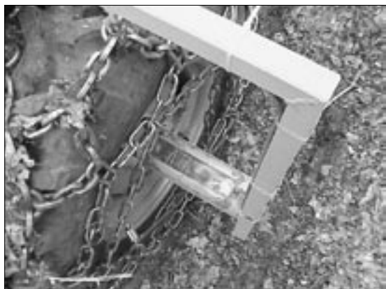
Figure 2: Sensor (rotation optical generator) mounted on wheel axle
