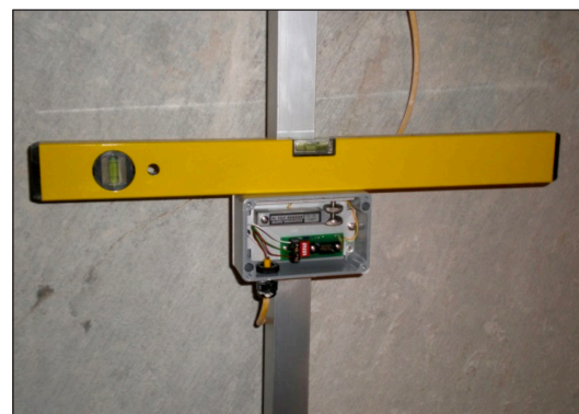
Figure 9. Safety Pillar VS3 (a) and Vertical EL beam gauge (b).
