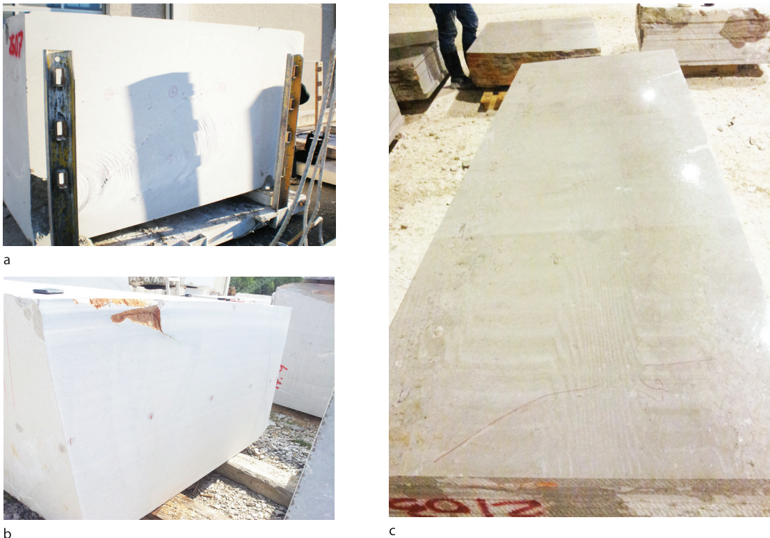
Figure 5: Measurement of the composed block (a, b) and review of the panels after cutting the block (c).
