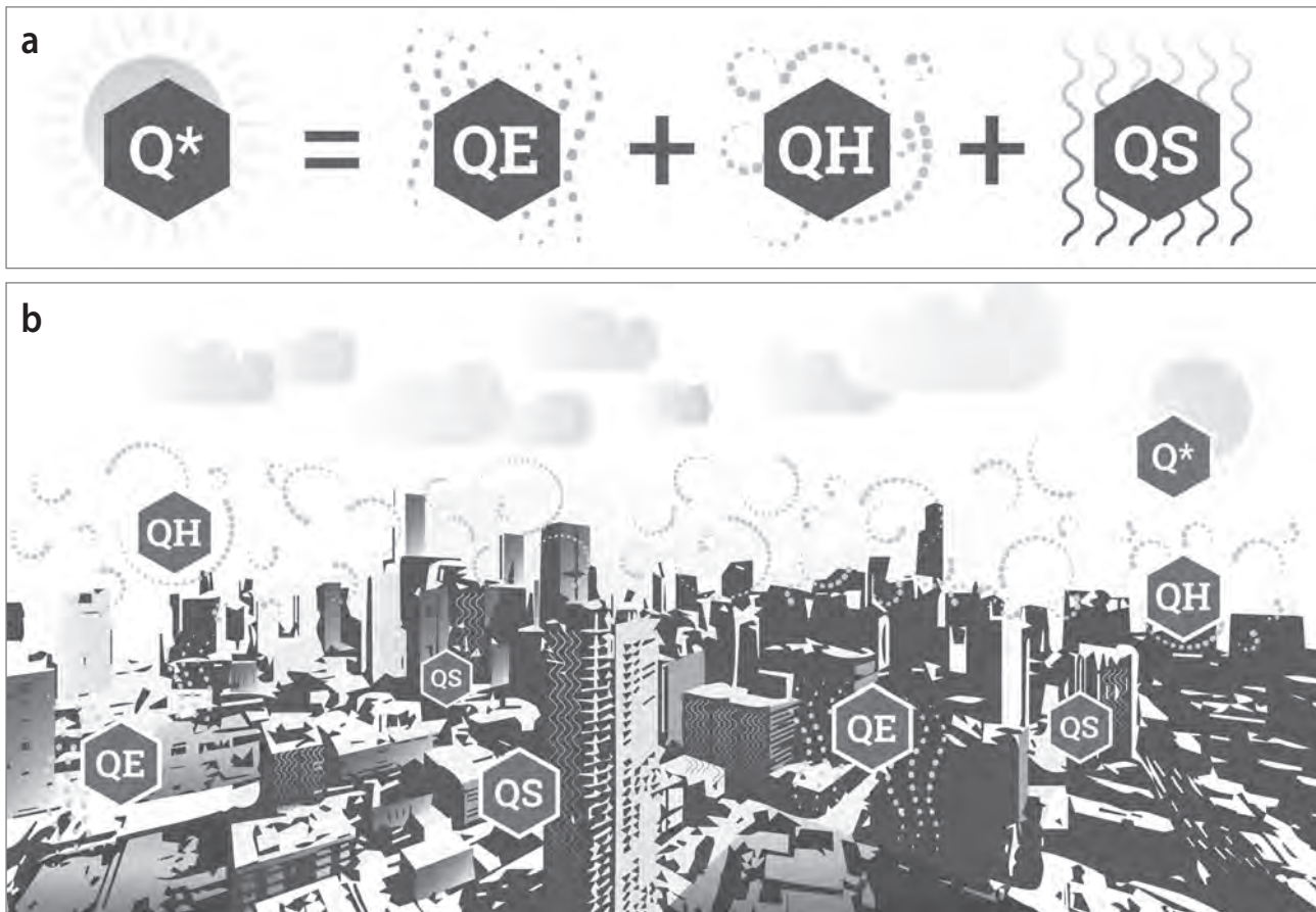
Figure 2: The surface energy balance in formula (a) and graphic (b) (author: Frank van der Hoeven).
