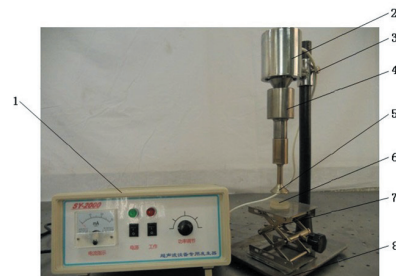
Fig. 9. Ultrasound standing wave levitation device; 1 ultrasonic-frequency power supply, 2 piezoelectric transducer, 3 adjusting screw, 4 amplitude transformer, 5 emitter, 6 reflector, 7 adjustment for the reflector and 8 fixed base
