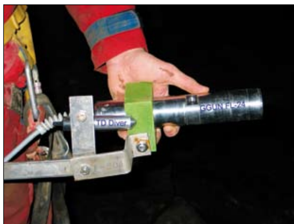
Fig. 5: Set-up of GGUN-FL24 and Schlumberger TD Diver fixed to a frame before the instalation to the river bank in Magdalena Jama (Photo: J. Turk).
