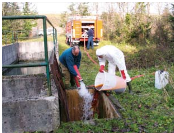
Fig. 4: Injection of Uranine into the oil collector at Ravbarkomanda (Photo: M. Petrič).
