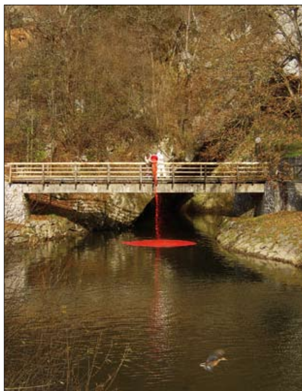
Fig. 2: Injection of Amidorhodamine G into the Pivka River at the ponor to Postojna Cave System (Photo: M. Perne).
