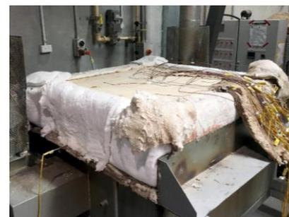
Fig. 4 Fire test set-up of floor specimens
