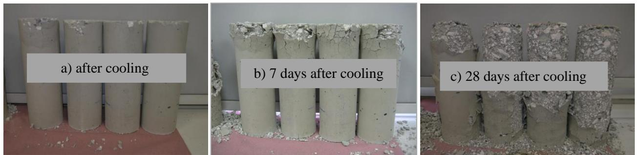
Fig. 1 The post-cooling appearance of reference concrete specimens heated to 800°C
