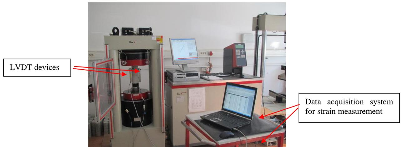
Fig. 1 Experimental setup – test machine and electronic equipment for compressive stress-strain monitoring
