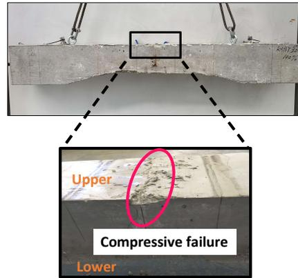
Fig. 7 Relationship between load and displacement Fig. 8 Compressive failure of Upper part in PC beam
