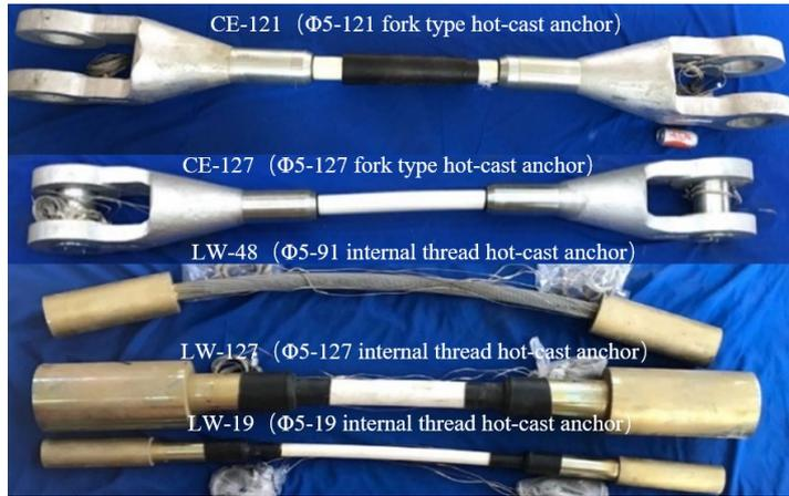
Fig. 2 Full-scale hot-cast anchors
