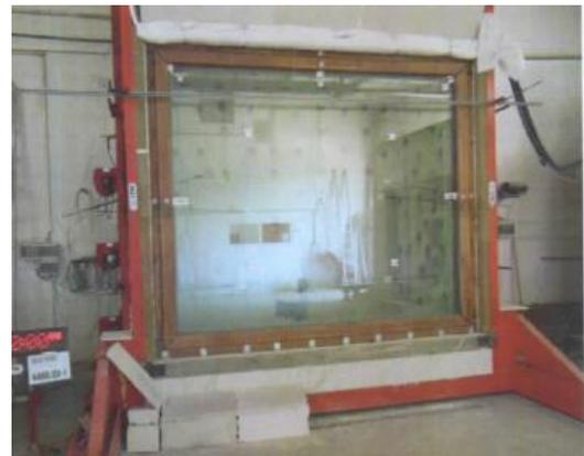
Fig. 2 Specimen preparation in the test furnace
