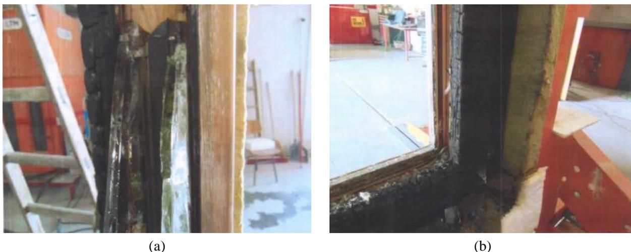
Fig. 8 Timber frame at the end of experiment: (a) unexposed or (b) exposed sides
