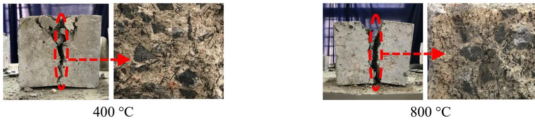
Fig. 6 Splitting tensile failure in HFRCs (HFRC2 as representative)
