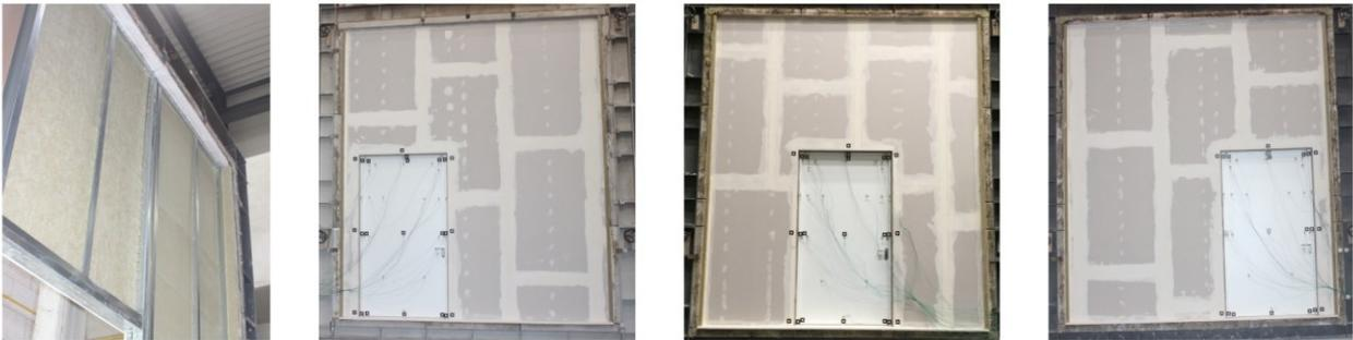
Fig. 3 Construction of the stud wall and test configurations (door placed at the left, middle and right position in the wall)
