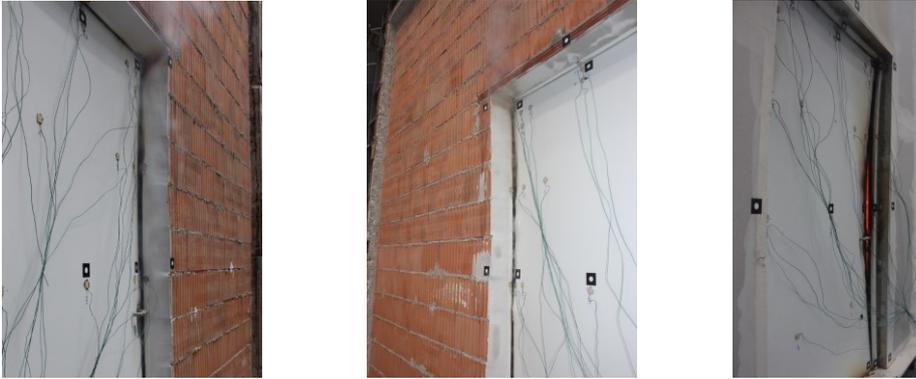
Fig. 6 Door deformation after 30 minutes: Door in the brick wall left position (left), in the right position (centre) and in the middle of the stud wall (right)
