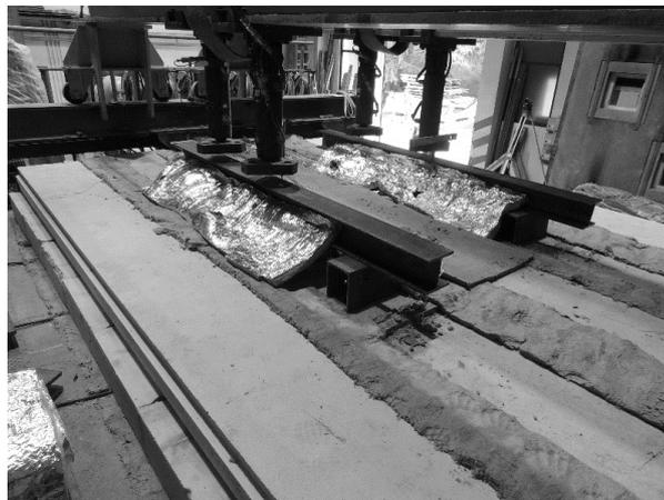
Fig. 2 Setup of the TCC beams over the horizontal furnace and loading equipment
