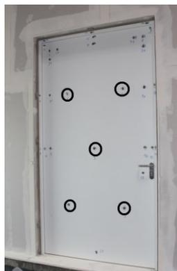
Fig. 1 Tested steel door embedded in the stud wall (temperature measurement positions are marked)
