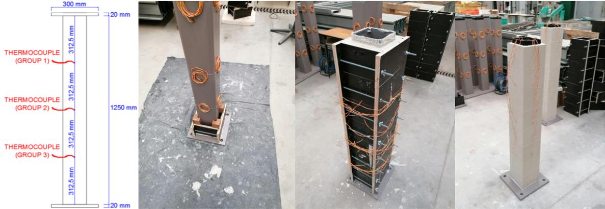
Fig. 1 Distribution of thermocouples and the different steps of casting mortars on the steel columns.
