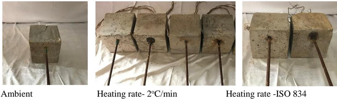
Fig. 6 Failure patterns of 12mm diameter rebar by following different heating rate
