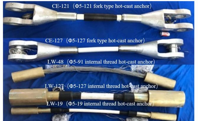
Fig. 4 Fire test specimens (Du et al. 2021)
