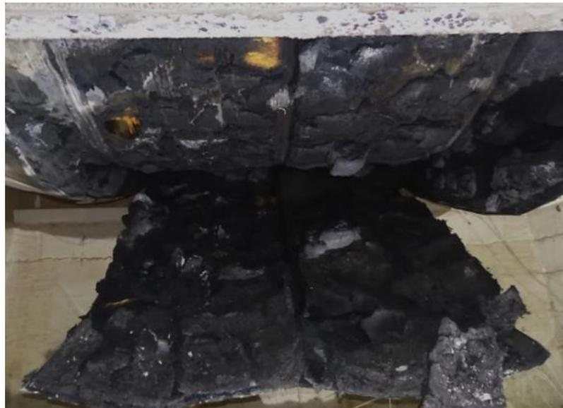
c) PIR foam core SP\_PIR\_160 after test
