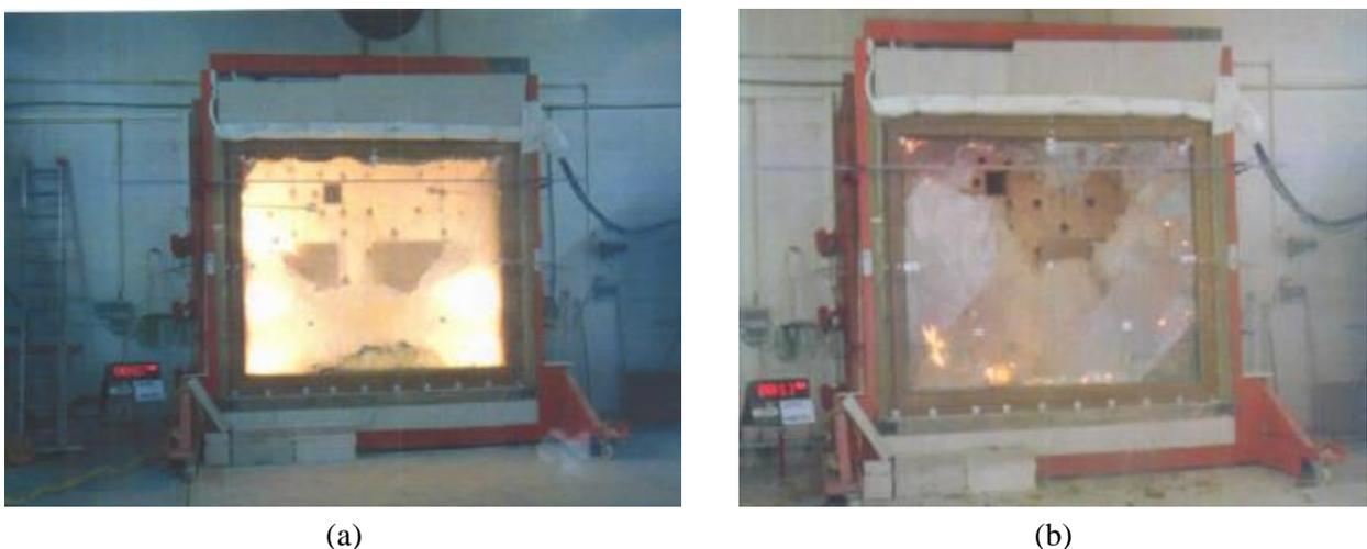
Fig. 7 (a) Cracking of the first layer of glass panel and (b) view of the specimen at the end of experiment
