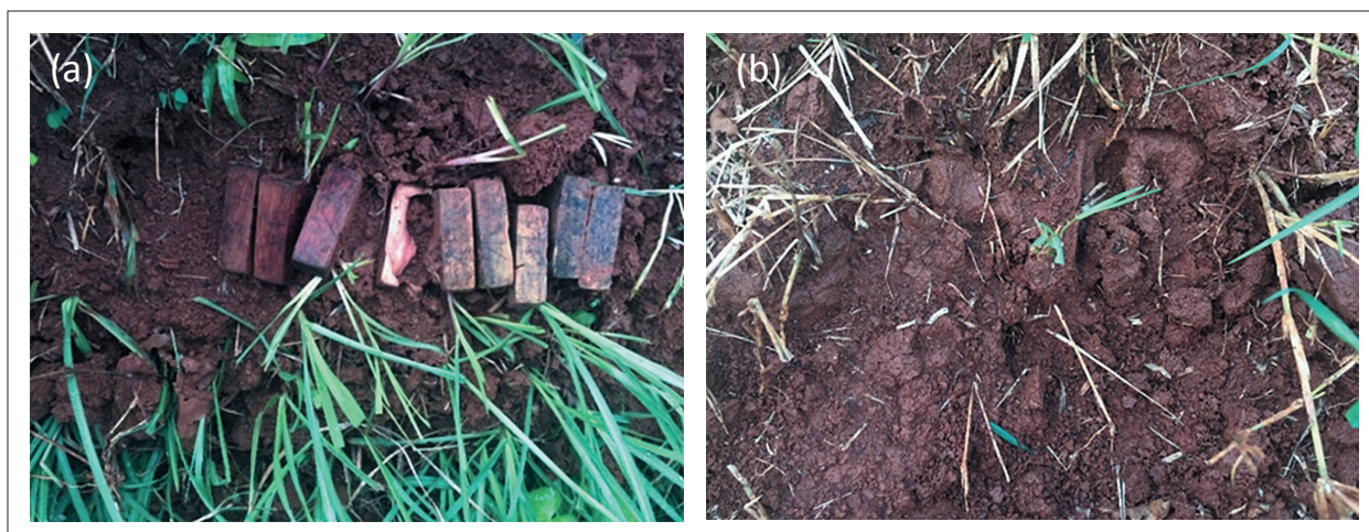
Figure 6. Sydney blue gum ( Eucalyptus saligna ) wood impregnated with Cu-EA and NO 50% (a) and NO 10% (b) after 16 weeks in a termitarium.
