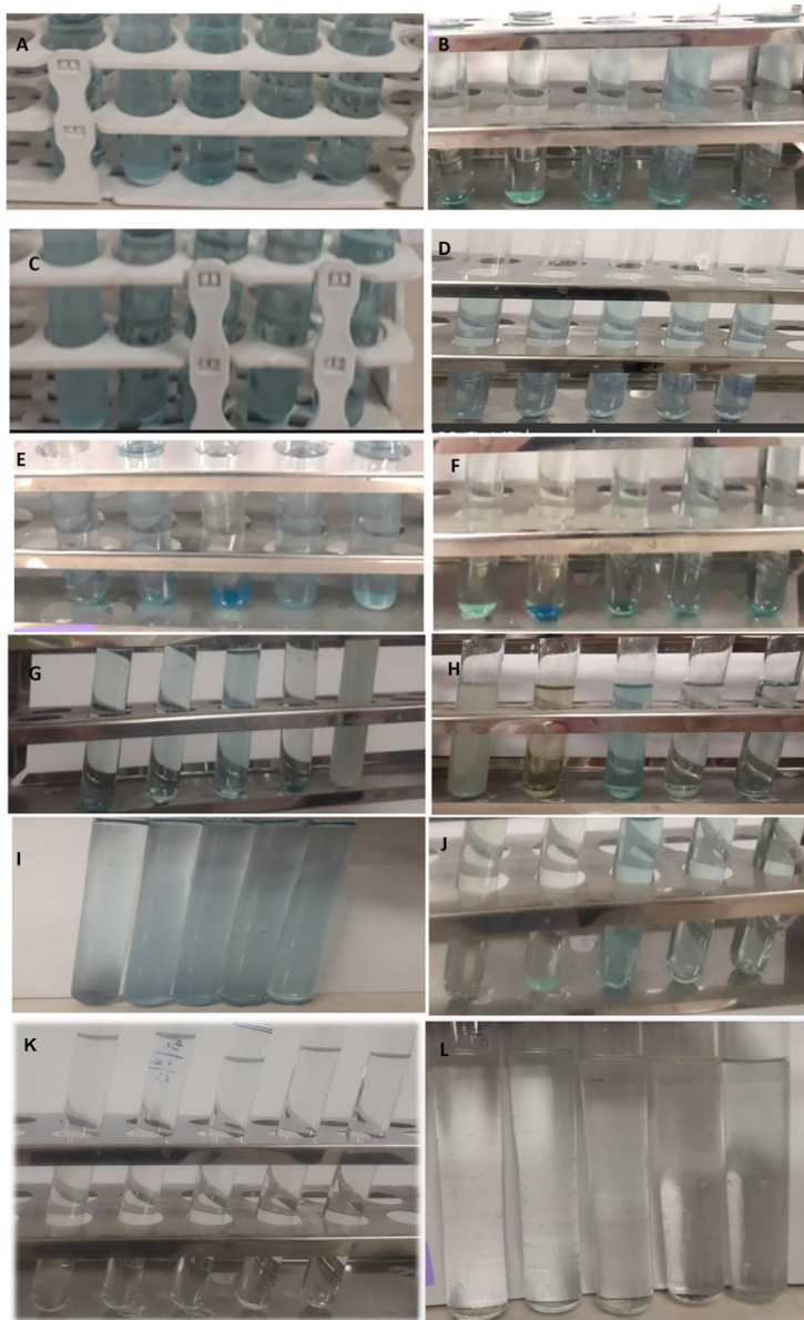
Figure 4: Coloured eluates of phycocyanin at different days and temperatures. A, day 3 / 5 °C; B, day 3 / 35 °C; C, day 5 / 5 °C; D, day 5 / 35 °C; E, day 10 / 5 °C; F, day 10 / 35 °C; G, day 15 / 5 °C; H, day 15 / 35 °C; I, day 20 / 5 °C; J, day 20 / 35 °C; K, day 30 / 5 °C; L, day 30 / 35 °C.
