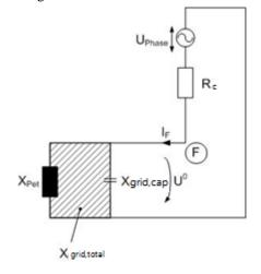
Fig. 16. Earth fault in an earth-fault compensated network; equivalent circuit
