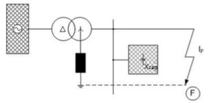
Fig. 15. Earth fault in an earth-fault compensated network; F ... fault location
