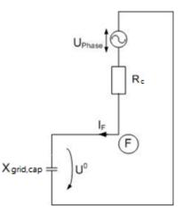
Fig. 13. Earth fault in a network with an insulated neutral - equivalent circuit; F... fault location
