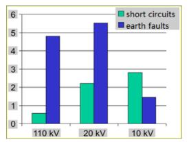
Fig. 1. Statistics for the single- and multi-phase faults, over voltage levels [1]
