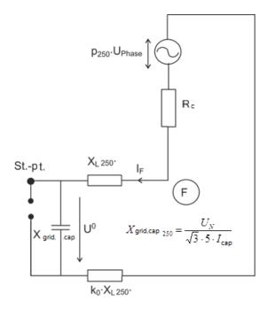
Fig. 17. Earth fault in an earth-fault compensated network; equivalent circuit
