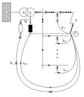
Fig. 18. Physical earth-fault current flow in a network with a resonance- and short-term resistance-grounded neutral point; F ... fault location
