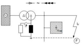
Fig. 19. Earth fault in a network with a resonance- and shortterm resistance-grounded neutral point -Electrical diagram; F ... fault location
