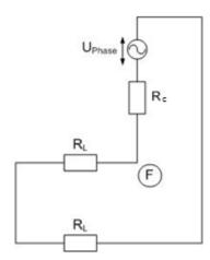
Fig. 6. Simplified representation of a ground fault in TN systems - equivalent circuit, F ... fault location
