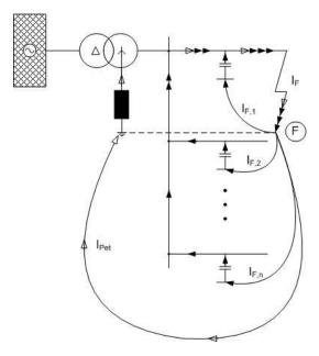
Fig. 14. Physical current flow for an earth fault in an earthfault compensated network; F ... fault location
