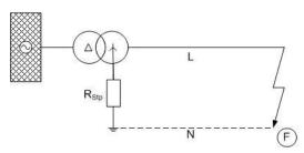
Fig. 7. Earth-fault in a resistance-grounded network - Electrical diagram; F ... fault location
