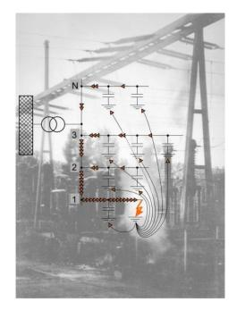
Fig. 10. Arc and capacitive earth-to-conductor current paths
