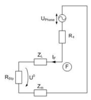
Fig. 9. Earth faults in a resistance grounded network - equivalent circuit; F ... fault location
