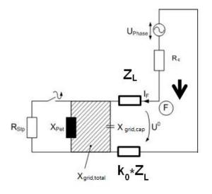
Fig. 20. Earth fault in a network with a resonance-g and shortterm resistance-grounded neutral point–equivalent circuit diagram; F ... fault location
