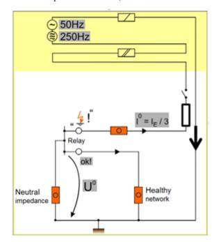
Fig. 3. Equivalent circuit for the single-pole fault with relevant parameters, [1]
