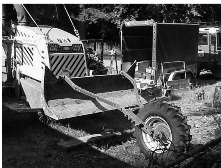
Fig. 2: Fifth wheel used on the front part of the tractor
