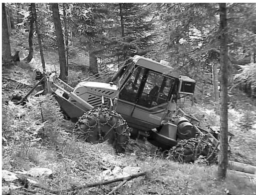
Fig. 1: Woody 110 tractor at a standstill, with the equipment for measuring technical parameters and the fifth wheel Slika 1: Traktor Woody 110 ob zaustavitvi z opremo za merjenje tehničnih parametrov in petim kolesom
