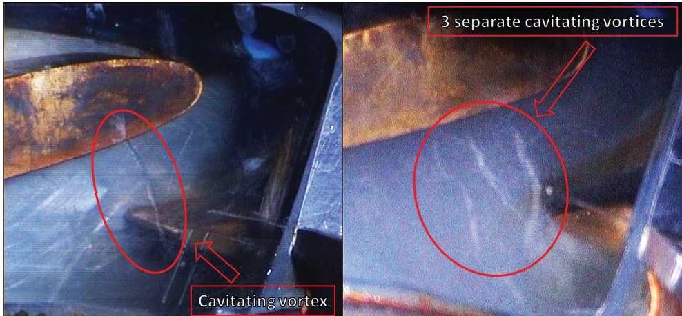
Figure 3: Cavitating vortices in the distributor region
