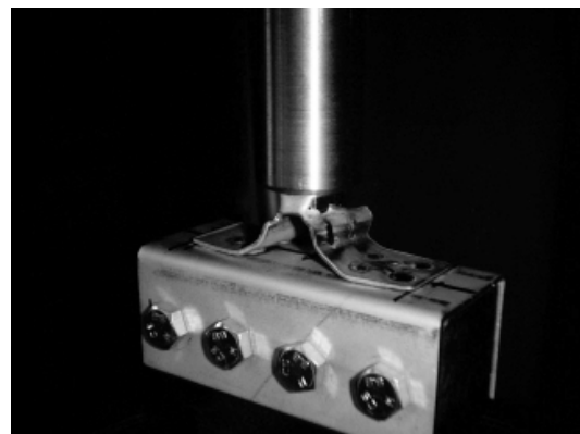
Figure 8: Static pulling test of holder
