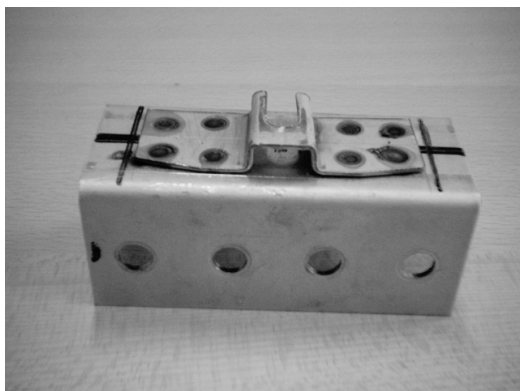
Figure 7: Holder welded by spots on pad for testing
