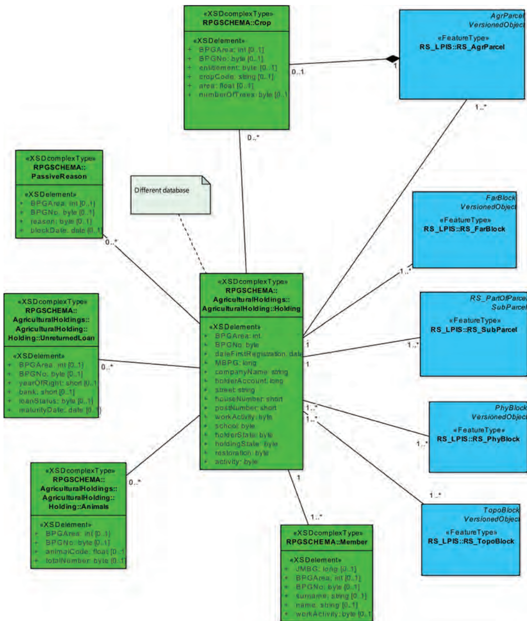
Figure 5: Connection between the registry of agricultural holdings classes and LPIS model classes.
