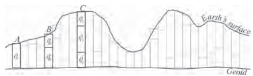
Figure 7: Division of right rectangular prisms per height to the smaller prisms.
