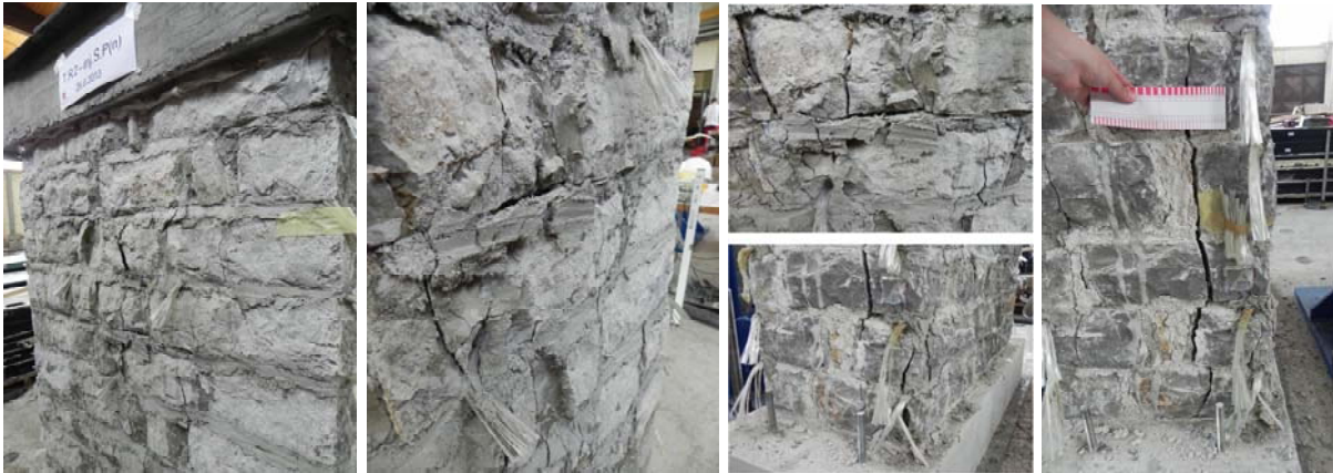
Figure 5.5: Damage pattern after failure attained at test T2 – I.S2.P (n) Slika 5.5: Poškodovanost zidu po testu T2 – I.S2.P (n)
