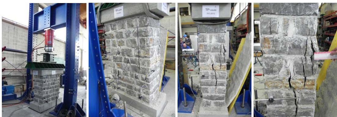
Slika 8.4: Postavitev tlačnega testa (levo) ter poškodovanost povezanega zidu po testu (ostale) Figure 8.4: Compression test setup (left) and damage of the wall with header stones after the test
