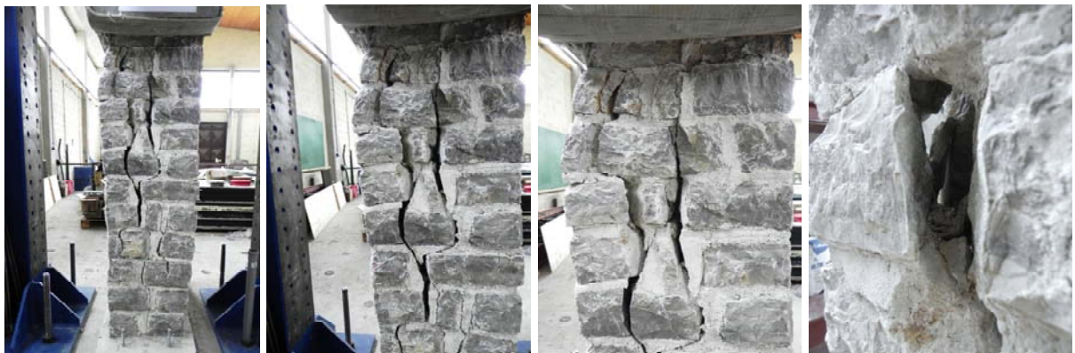
Figure 5.8: Leaf separation obtained at test T3-n Slika 5.8: Razslojevanje slojev zidu pri testu T3-n
