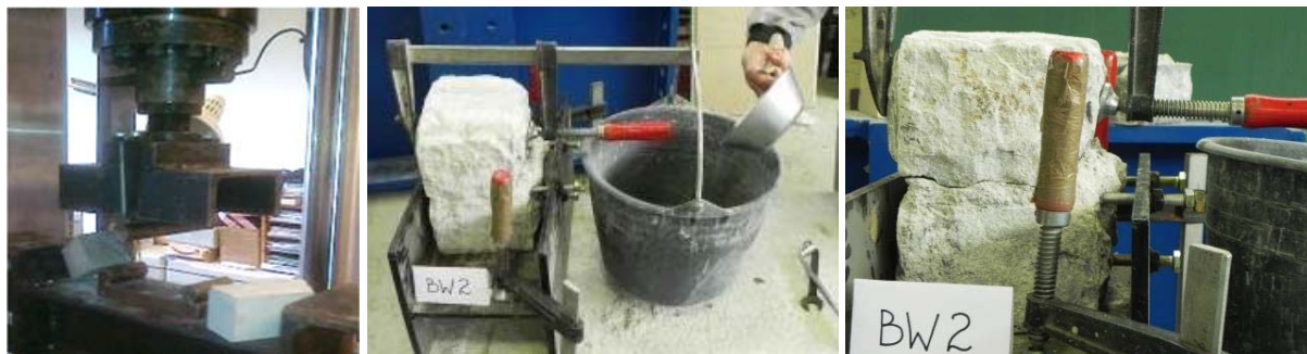
Figure 3.9: Three-point bending test of stone sample (left), “Bond wrench” test and mortar stone junction failure. Slika 3.9: Tri-točkovni upogibni test vzorca kamna (levo), “Bond wrench” test in porušitev stika malte in kamna
