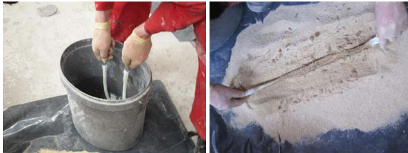
Figure 4.16: Impregnating the cord with an epoxy resin (left) and coating the cords in quartz sand (right) Slika 4.16: Namakanje vrvice v epoksi smolo (levo) in valjanje vrvice v kremenčevem pesku (desno)
