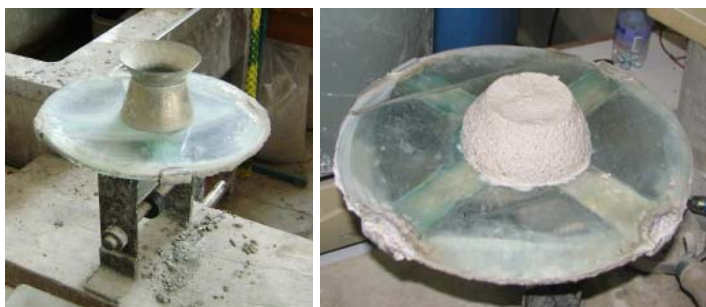
Figure 3.6: Mortar consistency test by flow table Slika 3.6: Preskus maltne konsistence na udarni mizici
