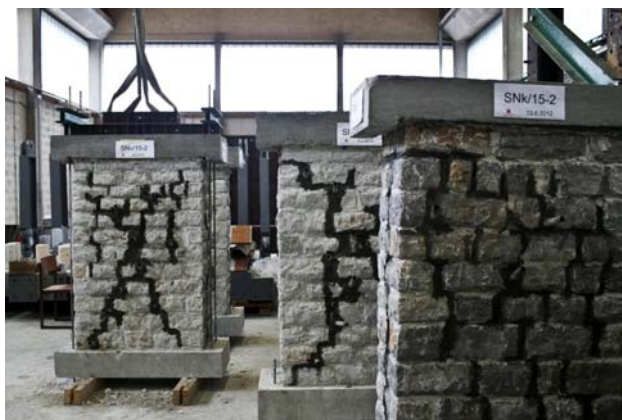
Figure 4.14: Grouted wall specimens (photo Željko Stevanić for UL FGG) Slika 4.14: Preizkušanci po linijskem injektiranju (foto Željko Stevanić for UL FGG)
