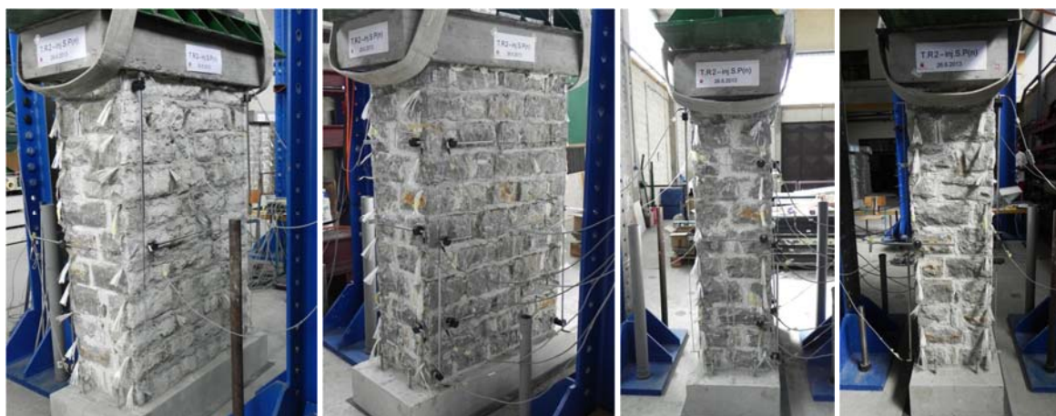
Figure 5.4: Grouted wall, additionally strengthened with NSM and transversally tied with glass cords (T2 – IS2.P (n)) prior testing (existing damage pattern)
