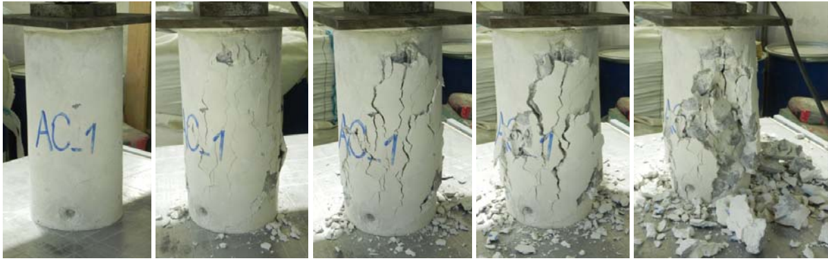
Figure 4.7: Failure mechanism of the cylinder during compressive test [251]
