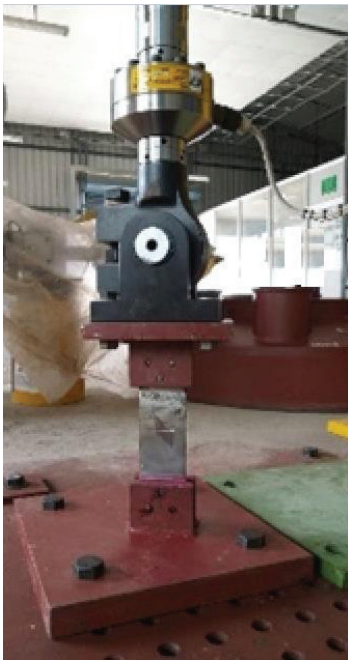
Fig. 11. Butt joint under fatigue loading
