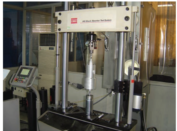
Fig. 1. MTS849 shock absorber performance test device used in the performance test
