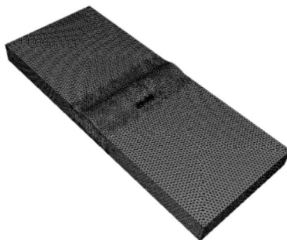
Fig. 8. Finite element model of butt joint
