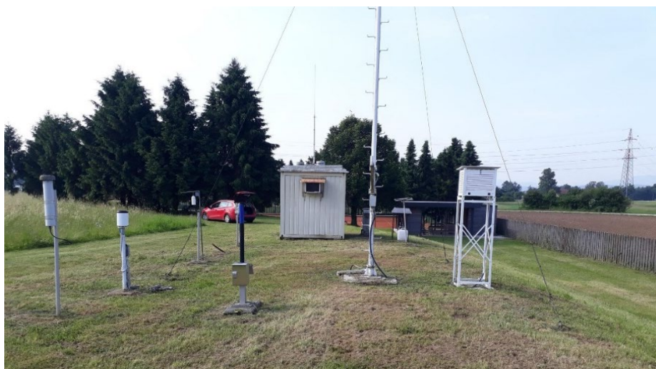
Figure 19: The Envinet Mira dose rate meter at the Ljubljana Brinje location
