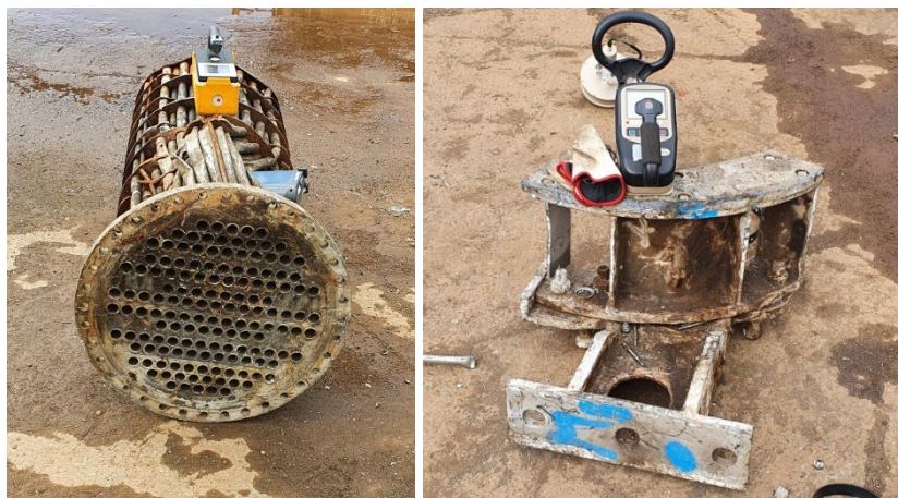
Figure 16: Two objects contaminated with ^{226}\text{Ra} in a shipment from Germany identified at the SIJ Acroni d.o.o. site (Photo: the SNSA Inspection)
