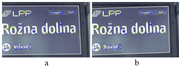
Figure 4. Detection of two targets on the same image using HIPs. Correct detection (a) has 58 matches, while wrong detection (b) has 60 matches.
