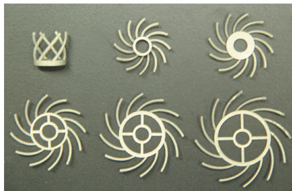
Fig. 6. Manufactured driving wheel and driven wheels
