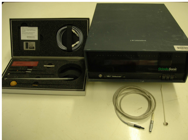
Slika 3.9 a) Inštrument za merjenje resonančne frekvence, b) sistem podpor. Figure 3.9 a) Apparatus for the determination of resonant frequency, b) support system.
