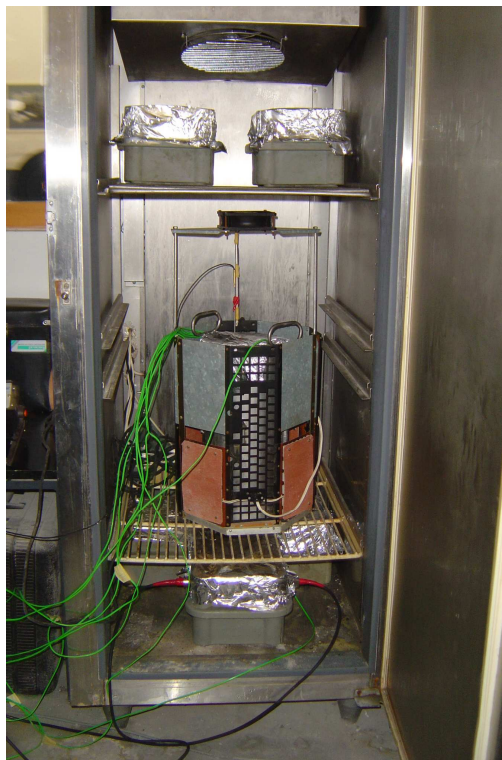
Slika 10.1 a) Uporabljen adiabatni kalorimeter, b) pripadajoča merilna oprema. Figure 10.1 a) Adiabatic calorimeter, used in this study, b) suitable PC equipment.
