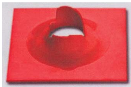
Slika 1: Videz prebite epruvete (vir: Thermoplastics Testing Center)
